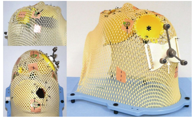
Figure 2 A phantom was used to evaluate the accuracy of the methods used to quantify the surgical pyramid. Three funnels were positioned inside a radiotherapy mesh plastic mask to simulate a total of five different surgical approaches: Small funnel, simulating a narrow and short approach; medium funnel (asterisk), simulating two different approaches, with the same superficial area and different deep areas, at distinctive distances from the surface; large funnel, simulating two approaches, with the same superficial area and different deep areas, at the same distance. Round, one-millimeter metallic markers were positioned over the mask as reference points for neuronavigation registration (black arrow). A reference frame (white arrow) was attached to allow the use of navigation systems (see text for further details).
