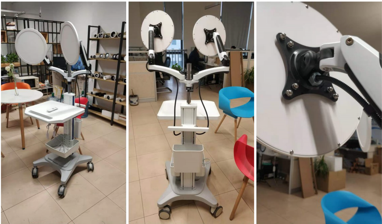
Figure 1 Twin beds removable bright light therapy apparatus. Front, back, and detail view.
