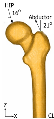
Figure 11 Boundary conditions applied in the healthy femur model.
