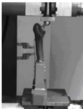
Figure 2 Illustration of testing model for axial load. The regular straight stem prosthesis was implanted into sawbones using bone cement. A Vancouver B1 fracture was then simulated and the construct was mounted on a testing device using a custom made angular stable fixation. Constantly increasing axial loading was then performed.
