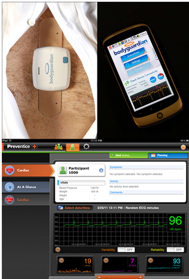
Figure 1 Remote monitoring system. Top left: The rechargeable module is attached to the adhesive SnapStrip. The SnapStrip is positioned vertically over the sternum. Top right: The cellphone serves as (1) a wireless communication hub with the cloud and (2) as a user interface. Bottom: Recorded physiologic data including ECG and heart rate are presented on an iPad for analysis and review. ECG: Electrocardiograph.
