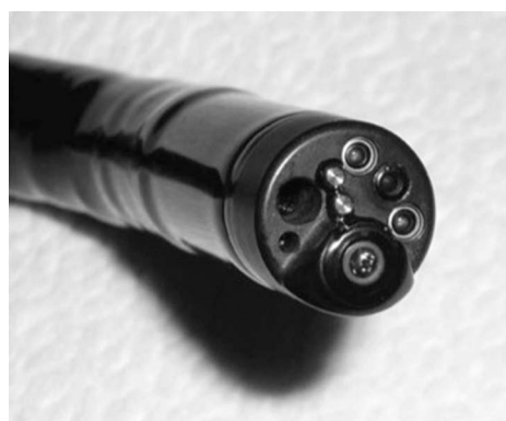
Figure 2 A confocal laser endomicroscope with a 5 mm diameter integrated in the distal end of a traditional colonoscope. Image from Dekker et al [1] (used with permission).
