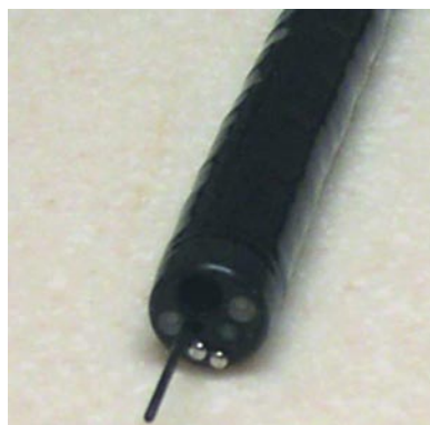
Figure 1 Image of fiber bundle extending through the biopsy port of a standard white-light endoscope [7] .
