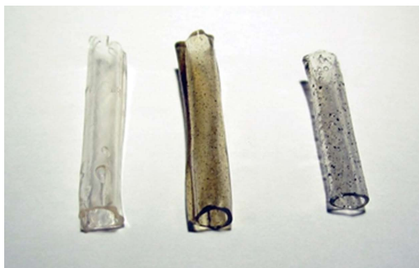
Figure 1 Synthetic biodegradable tubes of polyvinyl alcohol, polyvinyl alcohol loaded with COOH-functionalized multiwall carbon nanotubes MWCNTs (polyvinyl alcohol-carbon nanotubes, polyvinyl alcohol-carbon nanotubes tube-guides), and polyvinyl alcohol loaded with polypyrrole (polyvinyl alcohol-polypyrrole, polyvinyl alcohol-polypyrrole tube-guides).
