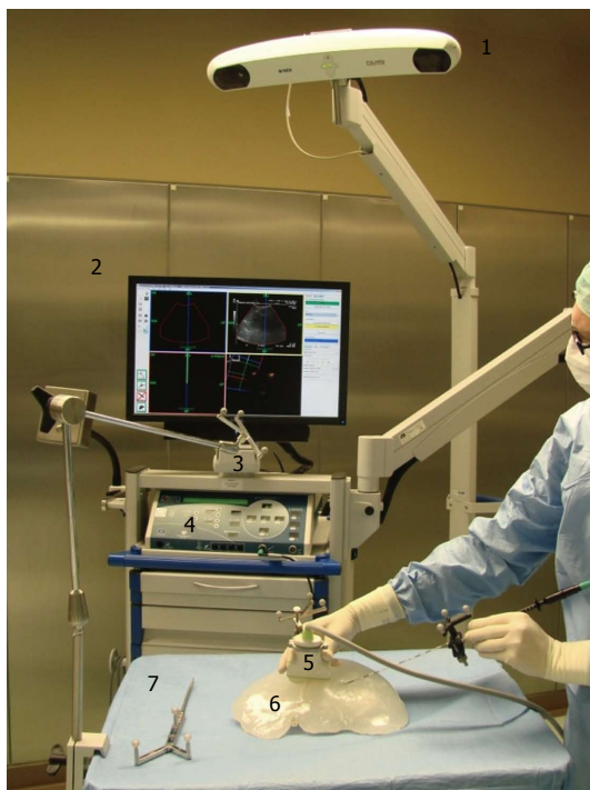
Figure 4 Example for a navigation device using optical tracking. The crucial elements are shown under intraoperative conditions with a phantom liver model. 1: Stereoscopic camera; 2: Monitor with a horizontally and vertically split screen; 3: Reference point; 4: Radiofrequency generator; 5: Ultrasound probe; 6: Liver phantom; 7: Pointer.
