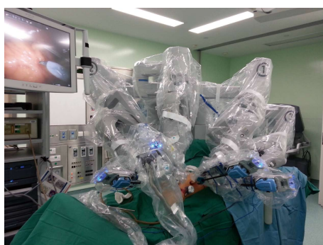
Figure 3 The 4-arm Da-Vinci Si robotic setup for low rectal cancer resection.
