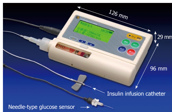
Figure 6 Newly designed wearable artificial endocrine pancreas. The total system is packed into a small unit (12.6 cm × 2.9 cm × 9.6 cm) weighing 250 g (KAP-003, Nikkiso). A glucose sensor is placed in the subcutaneous tissue and measures glucose concentration continuously. The blood glucose concentration (BG, in mg/dL) and the insulin infusion rate (IIR, in mU/min) appear every minute on a large LCD display.
