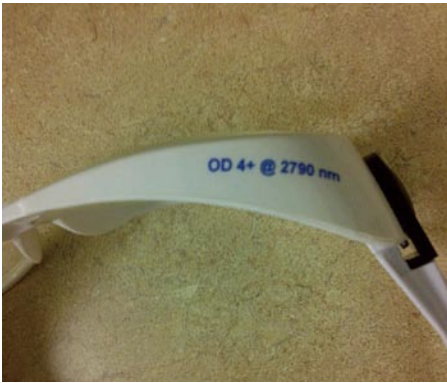
Figure 3 Optical density engraved on laser safety eyewear.
