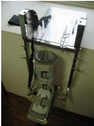
Figure 1 Knee rotation jig prior to mounting of specimen.
