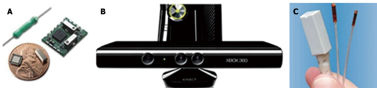
Figure 1 Various sensors which are commercially available [12] . A: Miniature magnetometers offer orientation and acceleration information, [Bertda Services (SEA) Pte. Ltd.]; B: Three-dimensional (3-D) range camera used in a widely commercial product; C: 3-D guidance system used in endoscopy devices (initiation).
