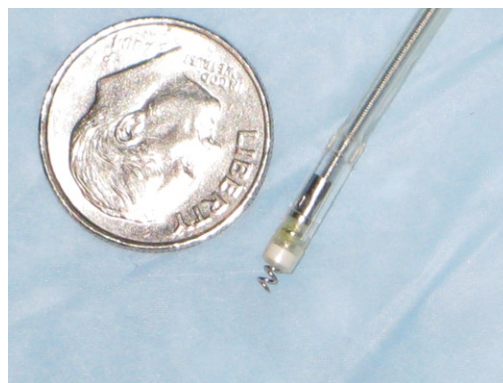
Figure 1 Stimulating electrodes. Two electrodes (Medtronic CapSureFix Model 5076) were used in this study. This model had an electrically active helix that was designed to extend easily (up to 2 mm) for active fixation and retraction. The electrodes were positioned at 15 cm and 12 cm above the anal verge.
