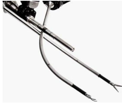
Figure 2 Robotic single port laparoscopic surgery module designed by Intuitive Surgical. ©[2015] Intuitive Surgical, Inc.
